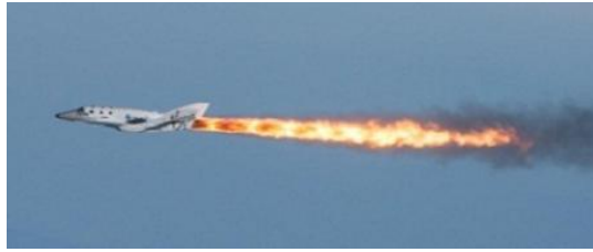
Figure 1: SpaceShipTwo with RocketMotorTwo firing ( http://www.parabolicarc.com/wp-content/uploads/2013/04/ss2_engine_firing.jpg . [Accessed 23 4 2014])
