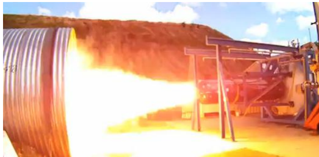
Figure 2: RocketMotorTwo undergoing ground testing ( http://www.parabolicarc.com/wp-content/uploads/2012/03/RocketMotorTwo_Firing.png . [Accessed 23 4 2014])
